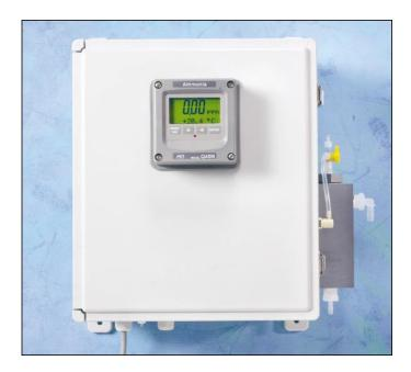
are 0-2 or 0-20 PPM, with a low end resolution of about 0.05 PPM. Response time to changes in ammonia concentration is less than 60 seconds to 90% of a step change in concentration, making the system much faster responding than competitive monitors. Two programmable alarm relays are available for local alarm functions, and two analog 4-20 mA output signals are provided for interface to plant DCS, telemetry, or other supervisory instrumentation.
